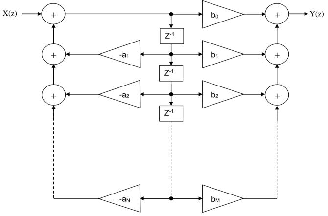
Direct Form-II structure is also known as Canonic Form realization. It is the modified form of Direct Form-I realization and it involves
