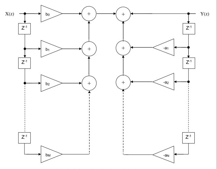
Direct Form-I structure is the basic form of realization and it involves
