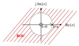
If the signal x(n) is right-sided with infinite duration, then its ROC is outside the circle of outer most pole.
