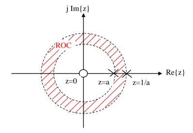
If the signal x(n) is both-sided with infinite duration, then its ROC is a finite duration ring, which lies between two poles.
