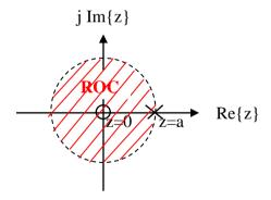
If the signal x(n) is left-sided with infinite duration, then its ROC is inside the circle of innermost pole.
