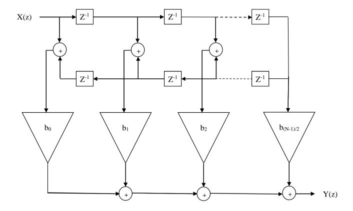
Linear Phase Realization of FIR system involves
